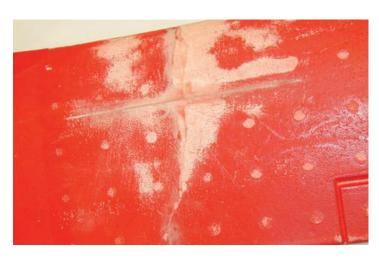
**Step 6:** Using fine sandpaper, sand the filler smooth and flush with the rest of the wing surface.
