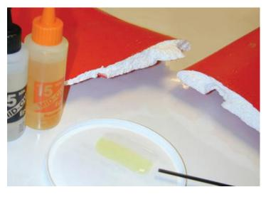
**Step 1:** In extreme cases, you might break a foam wing in two (or more!) pieces. A great trait of foam is that it is usually very easy to piece back together. Mix up a small batch of 15-minute epoxy on a plastic can lid. Run two or three lengths of each part as shown and then mix together.
