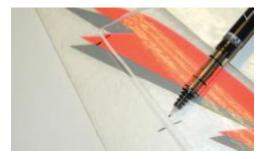
**Step 1:** It is not possible to repair a live-foam hinge, where the hinge is molded in as part of the control surface. It is best to install new hinges in the damaged surfaces. Before removing the surface, mark the locations for the new hinges. For this rudder, three 1/8-inch Robart Hinge Points will be installed.
