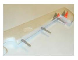
**Step 5:** Insert the Hinge Points into the holes, and set aside until the epoxy cures. Make sure that no epoxy gets into the pivot pins. If it does, quickly remove the hinge and install a new one. You have about 20 minutes before the epoxy starts to thicken and set.
