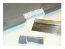
**Step 2:** If the dent is more pronounced, you can quickly cut away a section of the damaged material with a razor saw and glue in some new foam.
