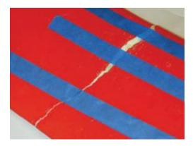
**Step 2:** Place some waxed paper or food wrap under the wing pieces and then apply just enough mixed epoxy to cover the exposed ends of the break. Use some masking tape to hold the parts together while they rest flat against your work surface. Be sure to wipe away any excess epoxy that oozes from the repair using a paper towel and some denatured alcohol.
