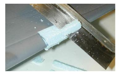
**Step 3:** Cut some new foam to length, and glue it in place with foam-safe CA. The best way to do this is to cut the foam a bit oversize, and spray foam-safe accelerator to the new material. Apply the CA glue to the cutout area, and insert the repair piece. Hold it in place until the glue sets. Use your saw to remove most of the unwanted material, then use a sanding block to smooth the replacement piece.
