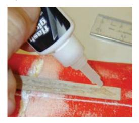
**Step 4:** If your wing is more than 36 inches in span, use a piece of thin plywood that is 4 to 6 inches long and ½ inch wide as an internal brace. Using a hobby knife and a razor saw, cut a straight line all the way through the wing, as shown. Test-fit the plywood, then apply foamsafe CA and insert it into the wing. Apply some accelerator, and let the glue set.
