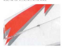
**Step 6:** Apply more glue inside the holes in the vertical fin, and slide the hinges in the rudder into place. Again, wipe away any adhesive that oozes out of the holes with paper towels and alcohol. Set aside until the epoxy sets.
