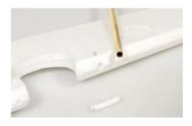
**Step 3:** Sharpen the end of a 1/8-inch brass tube, and use it as a drill to produce the holes for the Hinge Points. This produces much neater holes than a wood drill bit.
