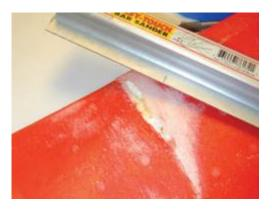
**Step 3:** After the epoxy has set, remove the tape. Using a sanding bar, smooth out the repair area.
